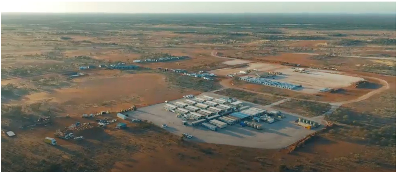
Figure 2: The SKA-Low construction camp site. Bottom centre is the “fly camp” or the camp built to enable other construction camp activities. The clear area to its left is the site of the final construction camp, and the clear area to the top right is the lay-down area.
